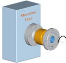
Type 11F Slow rotary movement with type 11F (1 fixed point, 1 side flexible)
