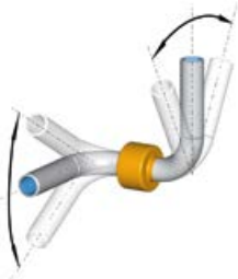
Type 13S Swivel movement on both sides with type 13S in angled pipe piece
