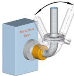
Type 12F Swivel movement with type 12F (1 fixed point, 1 side flexible)
