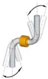
Type 13S Swivel movement on both sides with type 13S in straight pipe piece
