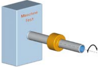
Type 11S Slow rotary movement with type 11S (1 fixed point, 1 side flexible)
